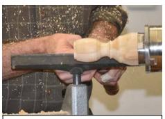
6. Defining the outside of the body. Starting to work toward the finished shape of the spindle bottom.
