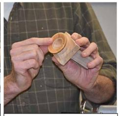
2. The underside of the roof is finished first, and sized to fit the top of the birdhouse body.
