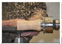
1. Start with a block about 2X the length of the finished body. Start forming it to a long oval with a spindle point.
