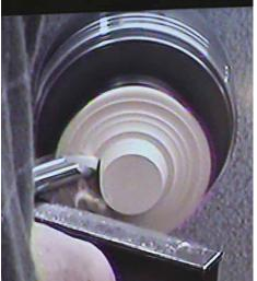
7. Shaping the outside of the roof.
